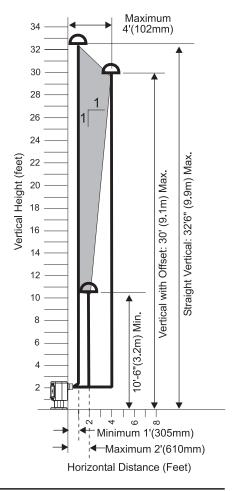
Vent restriction is required for certain venting installations, see the diagrams in "Venting Arrangment" section to determine if they are required for your installation.
